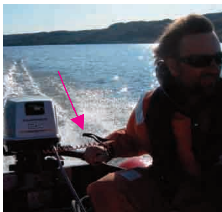
Figure 4.3 Operation from a 'dinghy' (rubber boat), illustrating the use of proper safety equipment, including a survival suit, a life jacket and the 'dead-man button' (red wire attached to the wrist).
